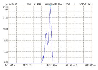
Typical Emission Spectrum at 50 mW Optical Power
