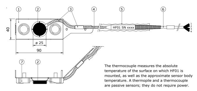
**Figure 2** heat flux sensor model HF01 with optional frame with magnets (2), connected to a high-temperature metal sheathed cable with interlocked spiral stainless steel armour (4) and low-temperature extension cable (6). The frame (1) with magnets (7) is an option intended for temporary mounting on carbon steel walls. It is provided with a cable strain relief (3). The armour may be electrically insulated by a silicone sleeve (5). Dimensions are in x 10<sup>-3</sup> m.
