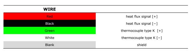
**Table 5.2.1** The electrical connection of a single heat flux and temperature sensor of an *RHF.* The shield is not connected to the stainless steel sensor body.
