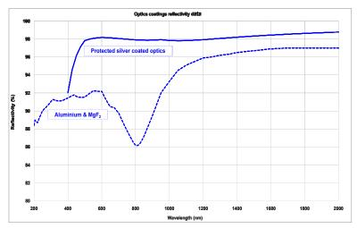
The graph shows the standard AI + MgF<sub>2</sub> optics coatings reflection efficiency versus wavelength.
