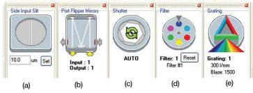
(a) Slit drive: Control the spectrograph slit width - drag blades on icon or type in required slit width
