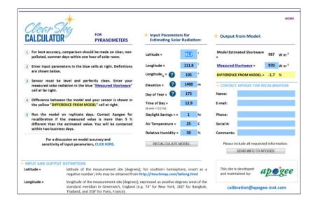
Clear Sky Calculator for pyranometers. Site data are input in blue cells in middle of page and an estimate of total shortwave radiation is returned on right-hand side of page.
