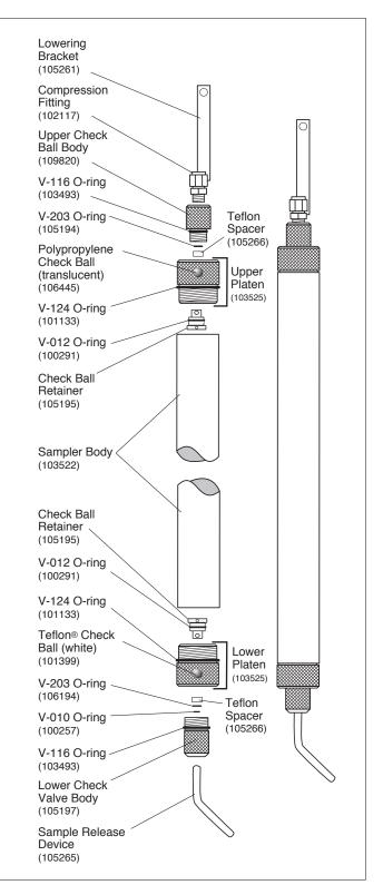
Model 425 1.66" x 2 ft. Discrete Interval Sampler (105264)
