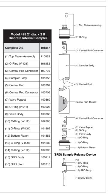
Model 425 2" x 2 ft. Discrete Interval Sampler (101857)
